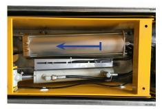
Remove the 4 circular head screws from MA6 from their respective vibrators and move the hydraulic pump to the left
