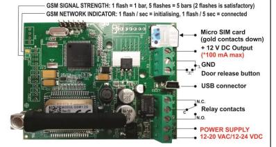
\*Do not use the 12V AUX power output for electric lock driving! You can use it to power external sensors: Short-term current load (up to 1 minute) - up to 500mA; Long-term current load up to 100mA! Use separate power source for door electric lock!
